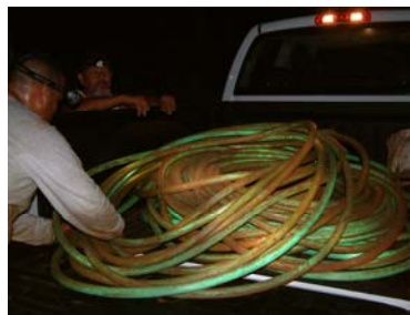
300 Feet of 3/4" spray hose
