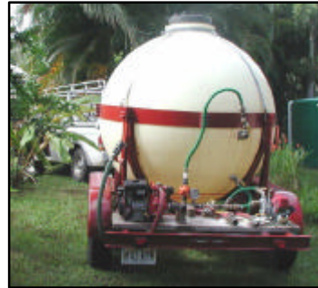
Spray tank apparatus used on the Big Island to control coqui
